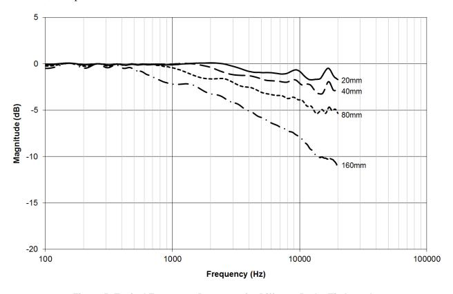
Figure 5: Typical Frequency Response for Different Probe Tip Lengths
