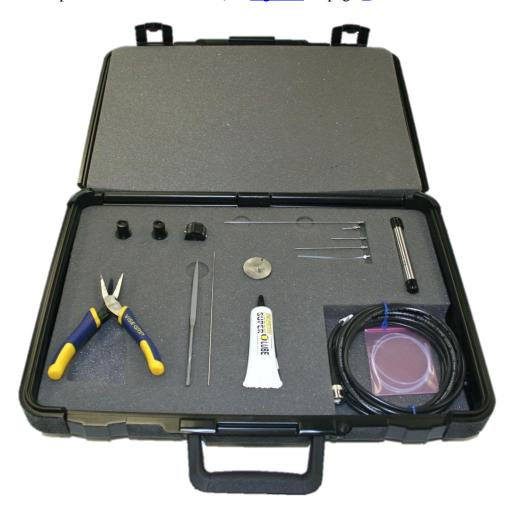
Figure 2: Probe Microphone Set
