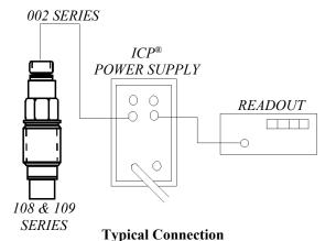
The figure above shows the 108 & 109 Series connected to a PCB Model 484B06 power unit. The 484B06 is a power unit that can be AC or DC-coupled.
