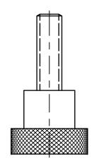
STANDARD CAMERA TRIPOD MOUNT (NOT SUPPLIED)
