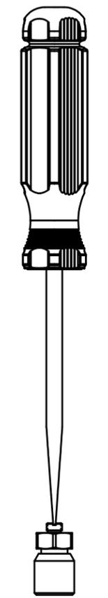
FIG 1: A 1/8" HEX ALLEN KEY IS REQUIRED FOR THE ENGLISH MOUNTING STUD. A 3MM HEX ALLEN KEY IS REQUIRED FOR THE METRIC MOUNTING STUD. APPLY SILICONE GREASE TO ALL MOUNTING SURFACES (SEE ARROWS FIG 1 & 2)
