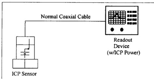
Figure 16. Sensor with Integral Electronics System Connector
