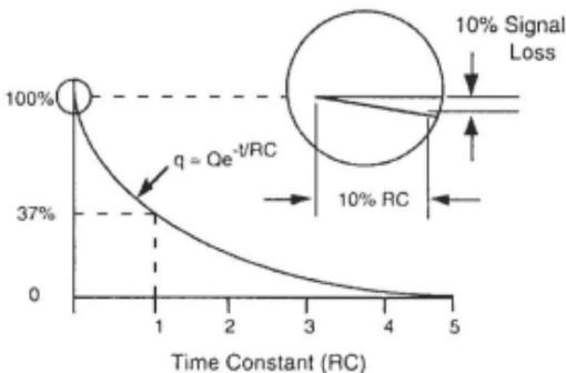
Figure 4 – Discharge Time Constant (DTC) Curve
