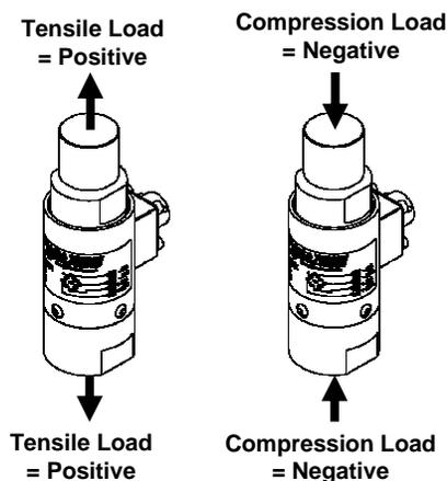
Figure 4 - Output Polarity
