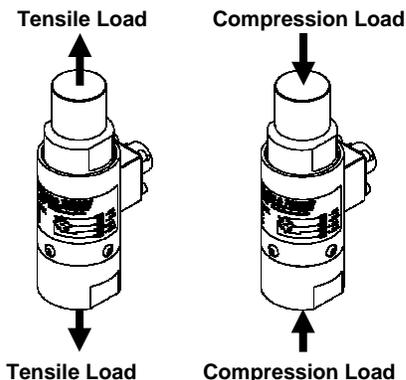
Figure 1 - Rod End Load Cell Loads
