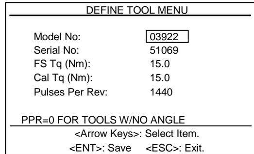
Figure 34 – DEFINE TOOL MENU Torque Screen
