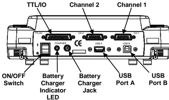
Figure 2 - Connector Panel
