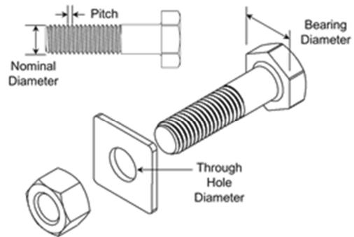
Figure 27 – Fastener Dimensions for Friction Calculations
