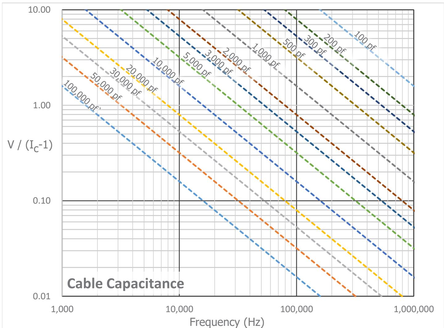
Figure 4: Cable Driving Nomograph
