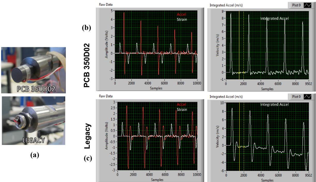
Figure 5. Shock at 50,000G peak with varying sensor models. PE sensor models with integrated mechanical isolators mounted on Hopkinson bar (a); integration to velocity of PCB Model 350D02 PE sensor (b); and integration to velocity of legacy PE sensor (c).
