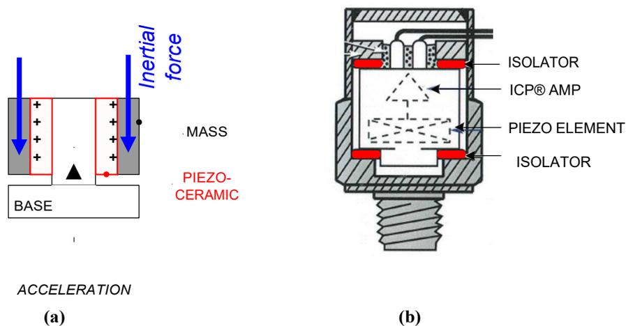
Figure 3. Piezoceramic element (a) and packaged sensor (b). Mechanical isolator isolates both the piezoceramic element and ICP® amplifier from out-of-band energy.
