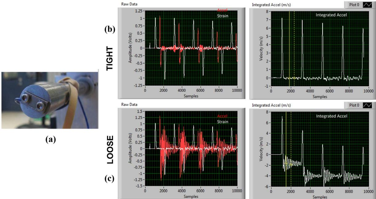
Figure 8. Shock at 50,000G peak with varying mounting torque. PCB Model 3991-60KG PR MEMS sensor mounted to Hopkinson bar (a); integration to velocity with proper mounting torque (b); and integration to velocity with inadequate torque on one of the two screws (c).
