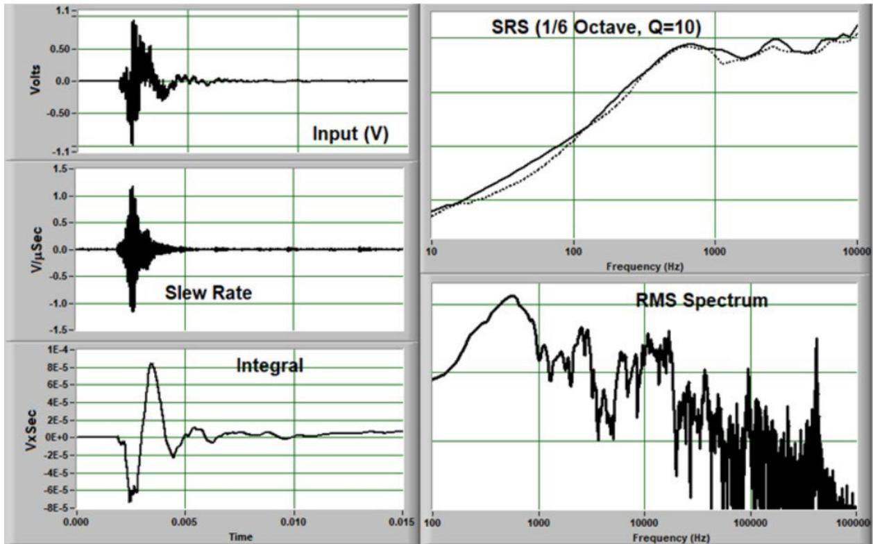
Figure 12. Shock Response Measured with an Endevco 7270
