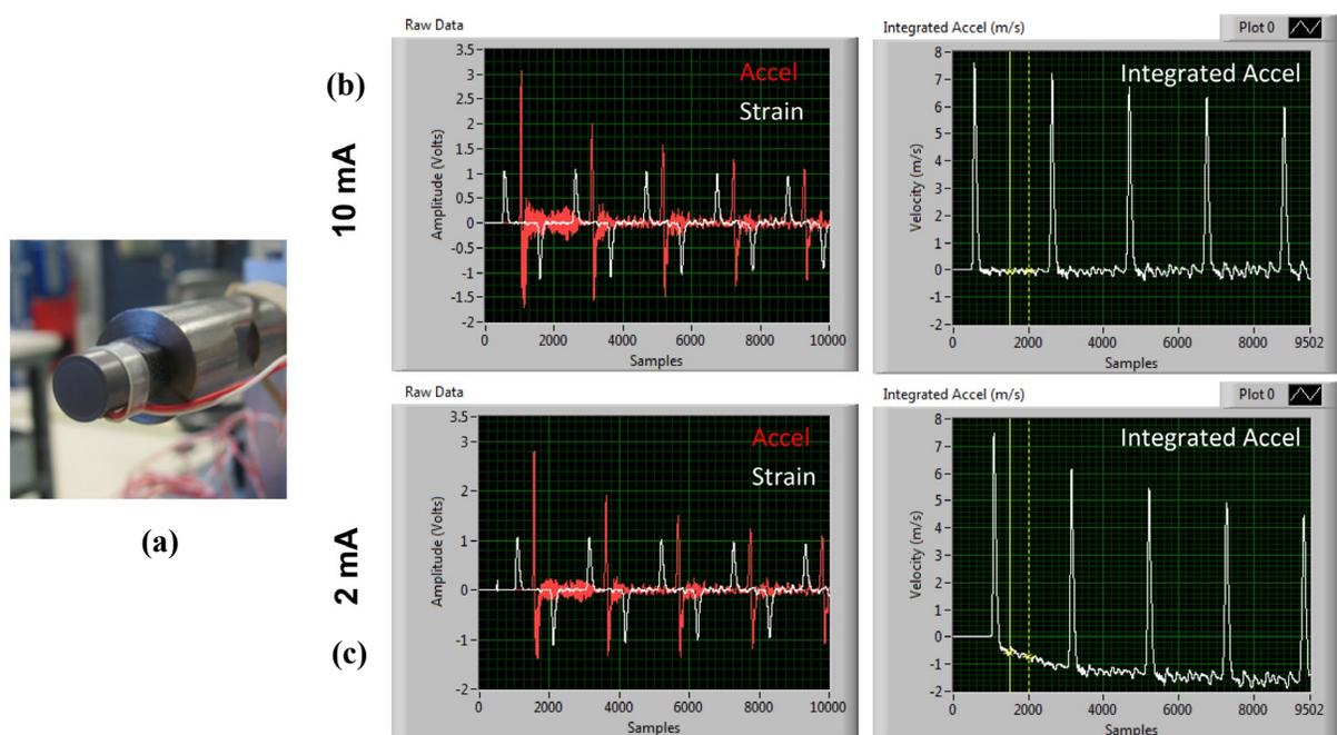
Figure 7. Shock at 60,000G peak with 130-foot long coaxial cable (4000 pF capacitance) and varying ICP® supply current. PCB Model 350B21 ICP® PE on Hopkinson bar (a); integration to velocity with 10 mA supply current (b); and integration to velocity with 2 mA supply current (c).
