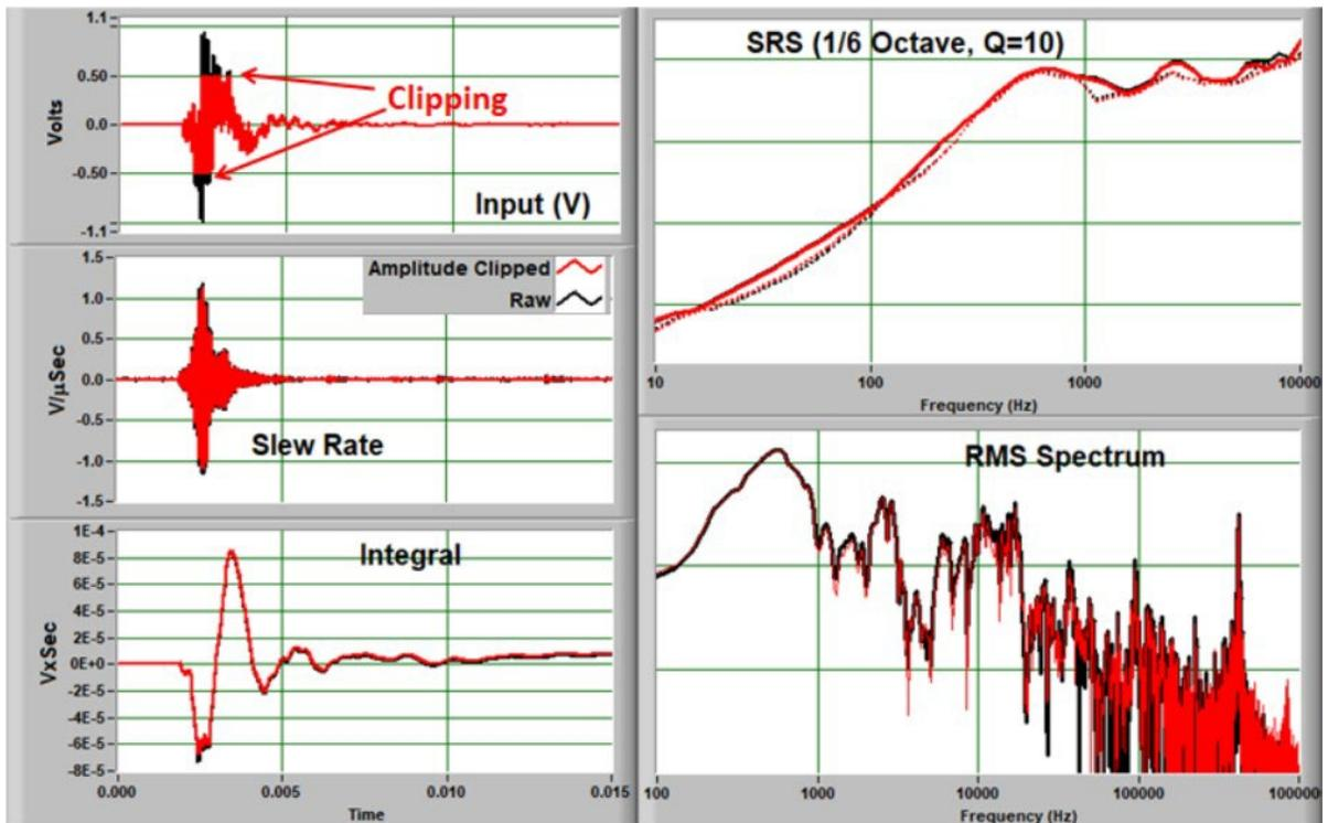
Figure 14. The Effect of 50% Amplitude Clipping
