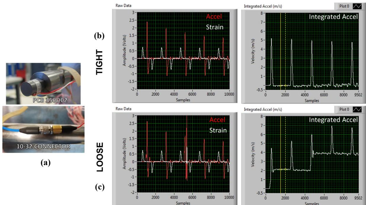
Figure 6. Shock at 28,000G peak with varying connection integrity. PCB Model 350D02 sensor mounted to end and cable/connector attached to the side of Hopkinson bar (a); integration to velocity with connector nuts tight (b); and integration to velocity with one of the nuts not fully engaged (c).
