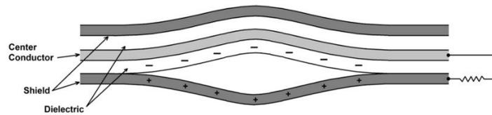
Figure 11. Charge Buildup Due to Cable Motion
