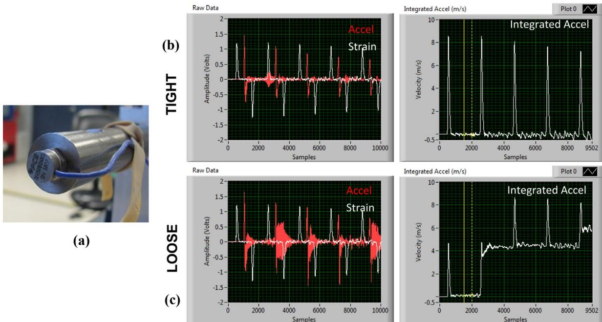
Figure 9. Shock at 50,000G peak with varying mounting torque. PCB Model 3501-50KG PR MEMS sensor mounted to Hopkinson bar (a); integration to velocity with proper mounting torque (b); and integration to velocity with inadequate torque (c).
