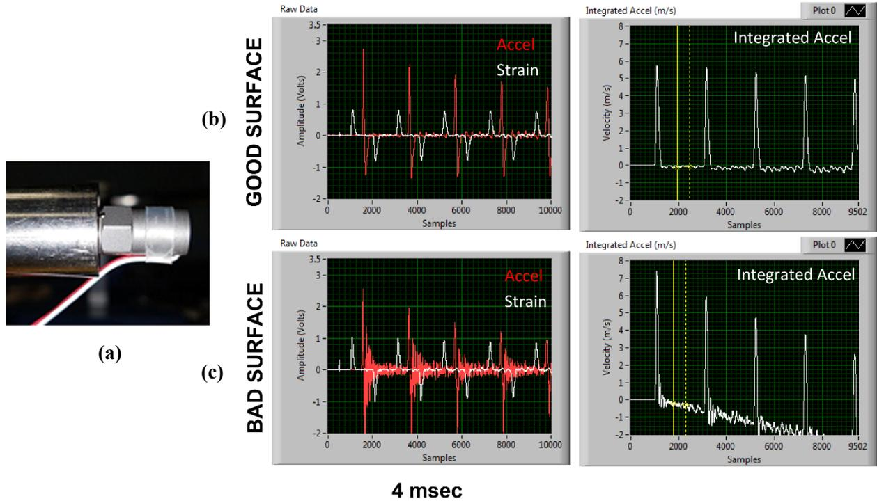
Figure 4. Shock at 25,000G peak with varying surface conditions. PCB Model 350D02 ICP® PE sensor on Hopkinson bar (a); integration to velocity with good mounting surface (b); and integration to velocity with 0.003-inch-thick debris on the mating surface at (c).
