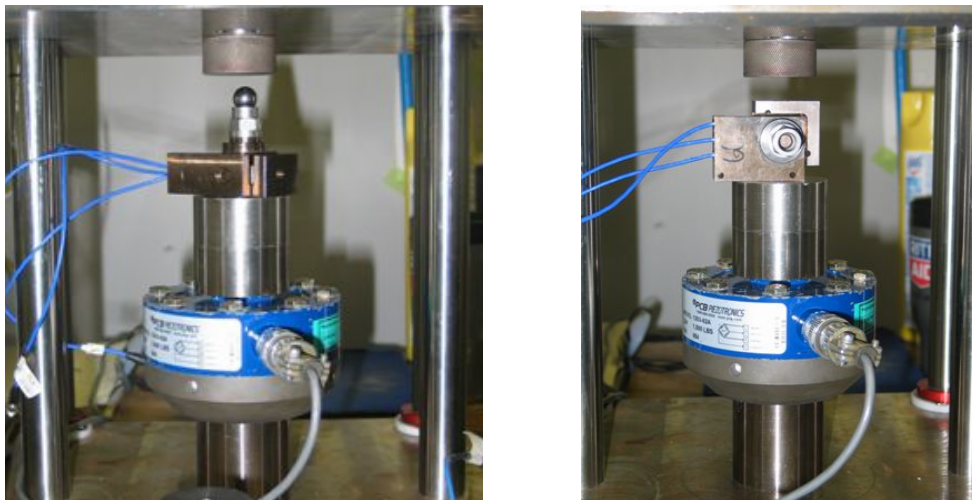
Figure 6 Shunt Method Calibration Z-axis Force Application through Threads (Left), X-Y Axis across Bolt (Right)
