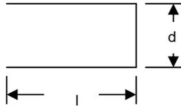
Using the speed of sound in air at STP,  $c = 1085$  ft/sec, or 13,021 inch/sec, the resonant frequency in the example above is 12.5 kHz. When Helium, a gas with less density leading to a faster speed of sound, is used for the calculation, the result is 36.7 kHz.
