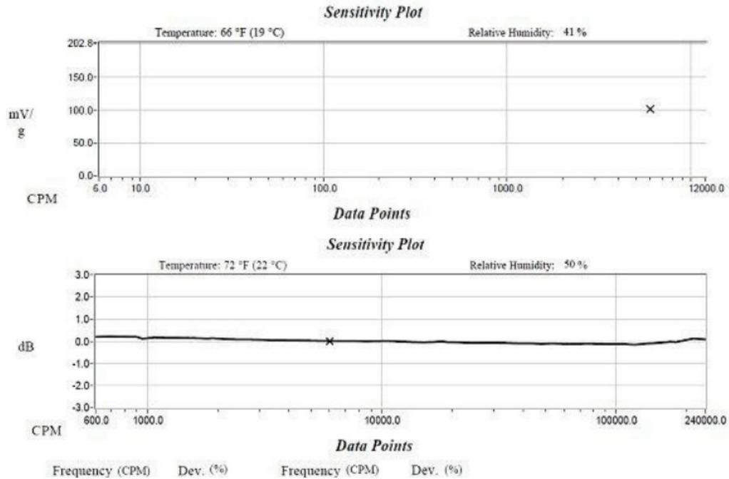
Figure 3: Comparison of calibration data for a low-cost (top) and precision (bottom) accelerometer
