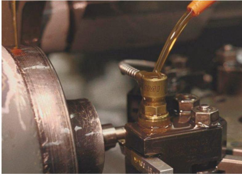
Figure 2: IMI 607A61 Swiveler® and armor-jacketed cable immersed in cutting oil
