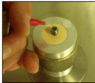
Figure 9B Leak Detection Test on Glass Bond
