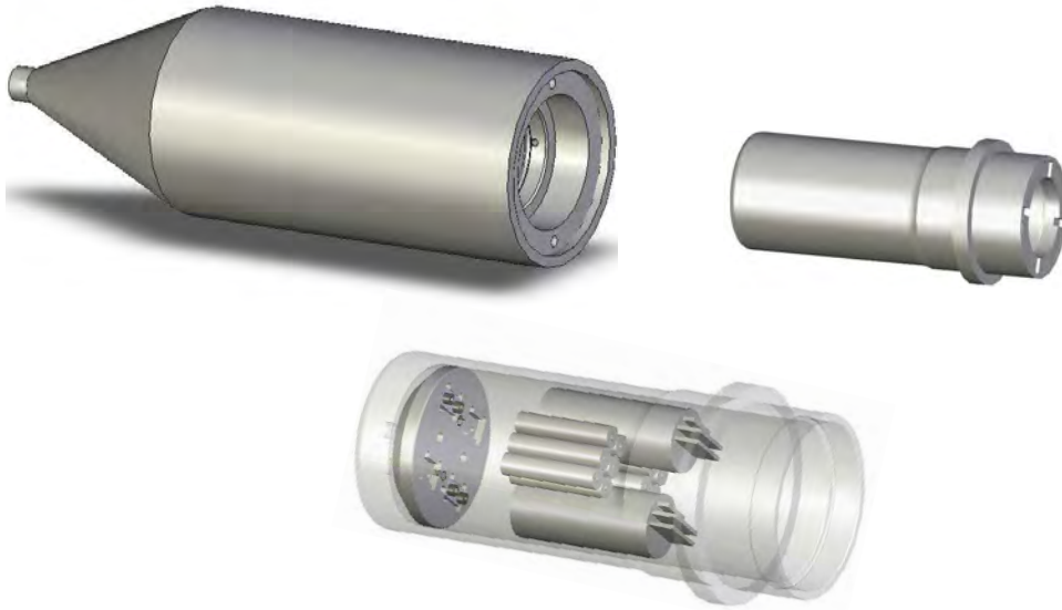
Figure 6. Configuration for test in STUBBI Penetrator. Two sensors were mounted in an instrumentation canister, along with batteries and recorders packed in glass beads. The recorders were set to 1MHz sample rate and 125kHz antialiasing filter. Illustration courtesy of A. Beliveau of Eglin AFB AFRL.
