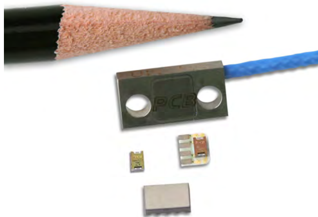
Figure 2. Scaled comparison of packaging configurations, shown approximately twice actual size. Above is the metal case with its cable, below that is the flip chip sensor and the substrate subassembly that can be used in hybrid chip and wire applications, and at bottom is the surface mount ceramic leadless chip carrier. Fixturing and techniques exist for determining sensitivity of all configurations.
