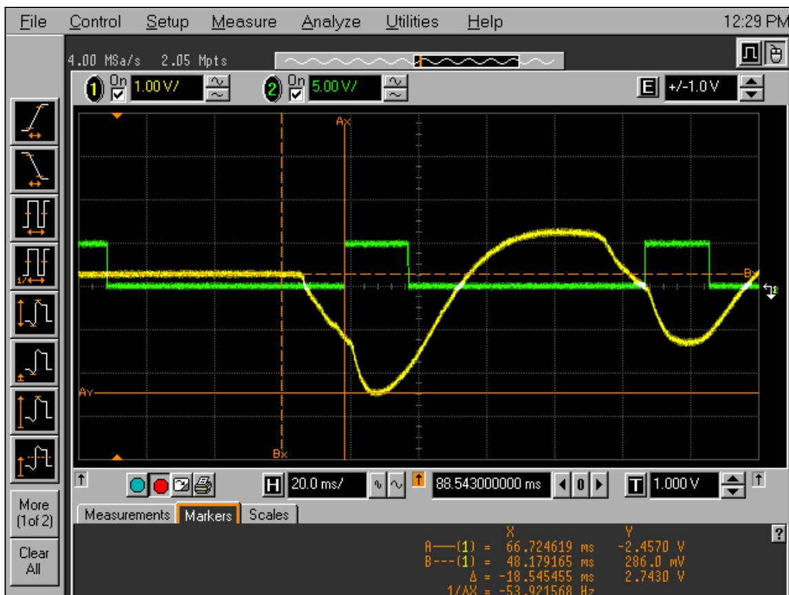
**Figure 1 – 113B28 Exposure to 4.6 BTU/ft<sup>2</sup>-sec for a duration of 18.54ms**
