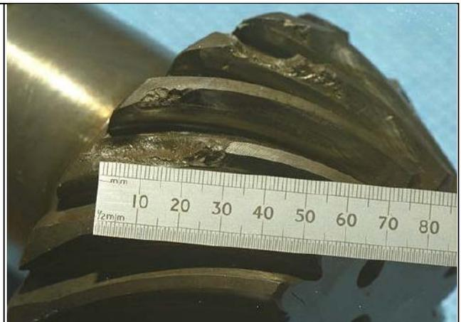
**Figure 3(b) A broken Gear Box Teeth**
