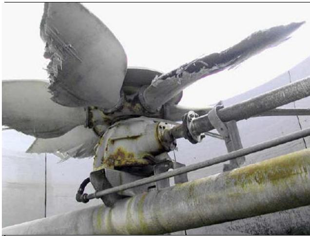
**Figure 3(a) A failed Cooling Tower Fan**
