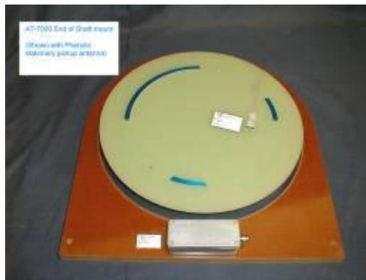
**End of Shaft [AT-7000](#) system for monitoring 16 Strain Gages and 24 thermocouples (on a different generator)**The AT-7000 multichannel system can measure RTD's, Thermocouples, Strain Gages, Pressure transducers, as well as differential Voltages (and Current shunts).
