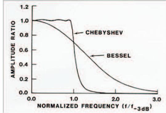
FIGURE 1A. COMPARATIVE AMPLITUDE RESPONSE
