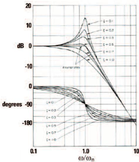
FIGURE 3. BODE PLOTS ACROSS CAPACITOR IN FIGURE 2
