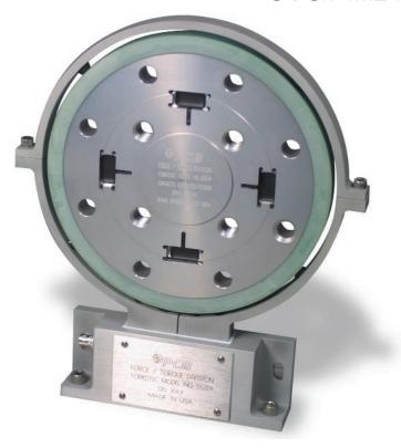
The Torkdisc® torque measurement system utilizes strain gage elements and digital, wireless telemetry to transmit data from rotating shafts. The Torkdisc® is very thin compared to other rotating torque measuring devices, permitting installation in areas where space is at a premium. With no bearings or other moving parts, the Torkdisc® offers exceptional longevity.
