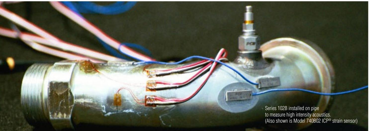
Series 102B installed on pipe to measure high intensity acoustics. (Also shown is Model 740B02 ICP® strain sensor)
