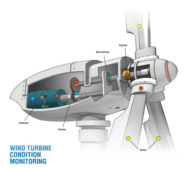
Some of the world's largest wind farms rely on IMI Sensors to keep their wind turbine operations at optimal performance by increasing reliability and reducing downtime. A broad range of industrial grade sensors from PCB<sup>®</sup> measure vibration, strain, torque and noise in new and existing wind turbines, providing measurements that are crucial to keep the operating health of these systems in tip-top shape.
