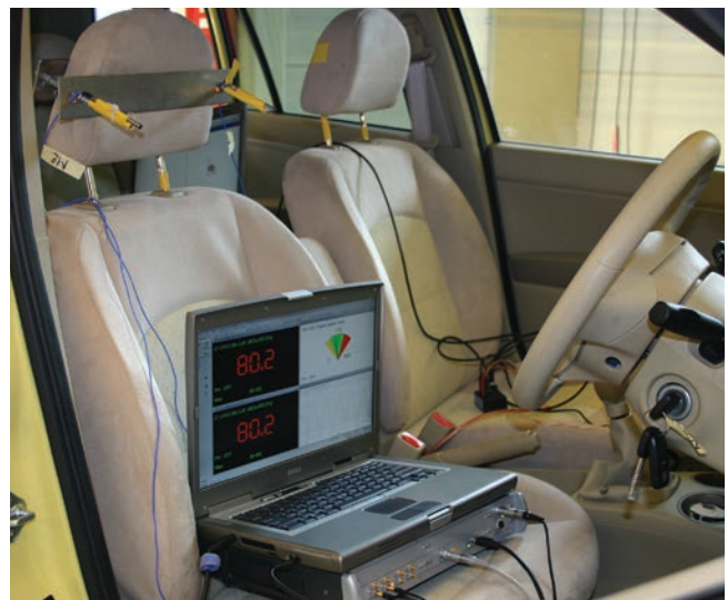
Cabin Noise Measurements for Rider Comfort
