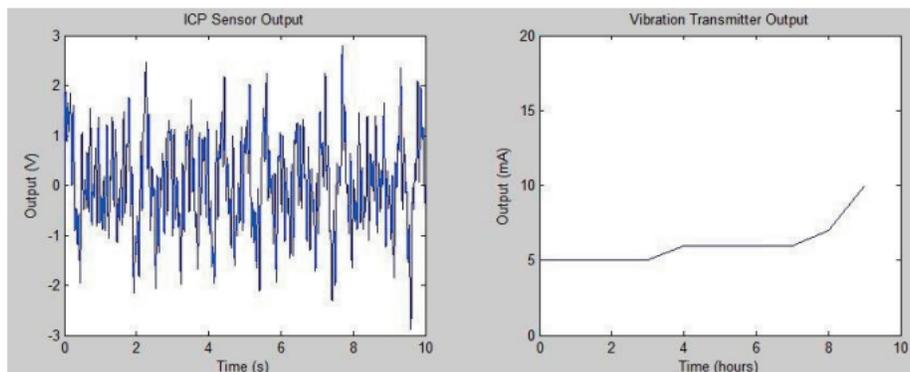
Figure 1: Comparison of ICP® sensor and 4-20 mA transmitter outputs
