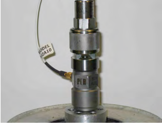
Figure 1: Frequency response test setup
