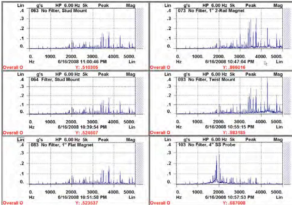
Figure 5: Acceleration spectra to 5000 Hz have significant differences
