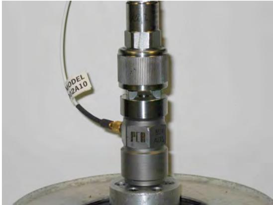
Figure 1: Frequency response test setup
