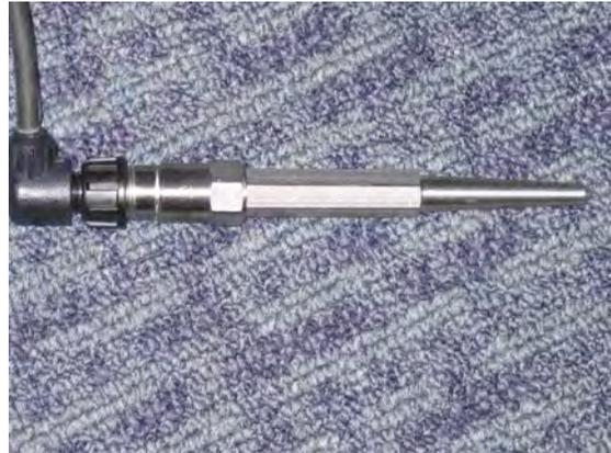
Figure 2: Stainless steel probe (stinger)
