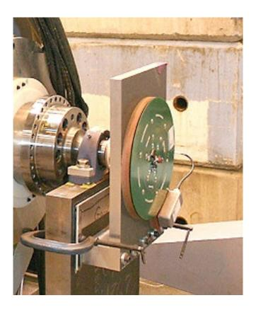
The picture above-left shows the rotating Transmitter for the 8 RTD's on the lower left, the stationary induction power/data Pickup on the lower right, and the Receiver (digital to analog output device) in the background. The above-right picture shows the system in action. The unit was able to operate properly despite extreme EMI from high energy 18 pole variable frequency drive electronics.
