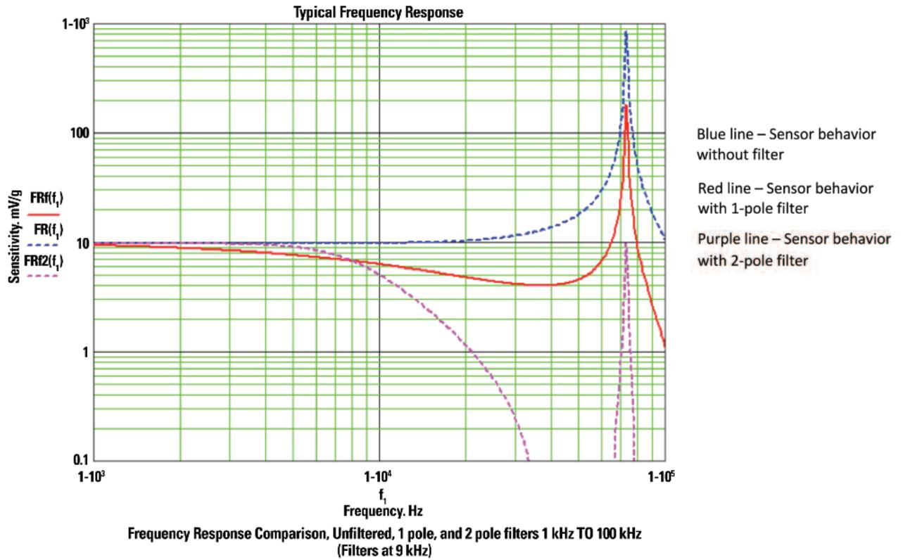
Figure 3 – Unfiltered and Filtered Sensor Response
