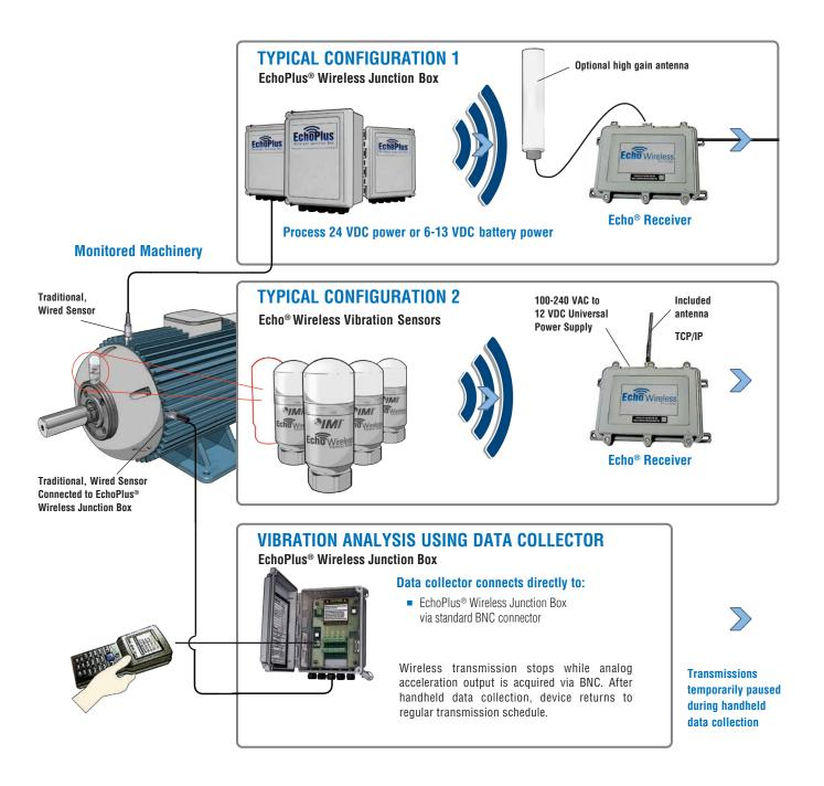
The Echo® Wireless Vibration Monitoring System is simple in design, easy to install, cost-effective and flexible in configuration. With over 400 points per receiver, the system can monitor over 3,500 points even within the same RF coverage area. Outside the same coverage area, the number is even higher. Stand-alone Echo® Sensors and EchoPlus® Junction Boxes can be mixed and matched as desired.
