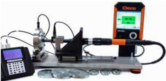
Basic Fastener Drive Systems are used with Model 962 or Model 3210 recorders and are controlled by the operator
