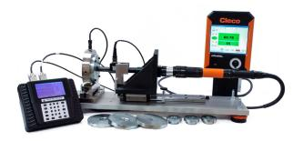
Basic Fastener Drive Systems are used with Model 962 or Model 3210 recorders and are controlled by the operator
