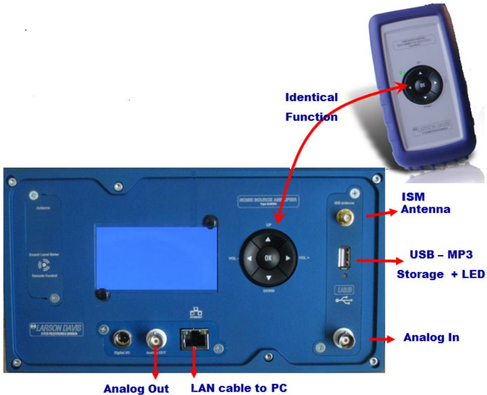
**FIGURE 3-1 BAS002 Power Amplifier Front Panel**
