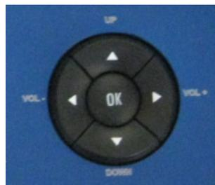
**FIGURE 3-4 BAS002 Amplifier Keypad**
