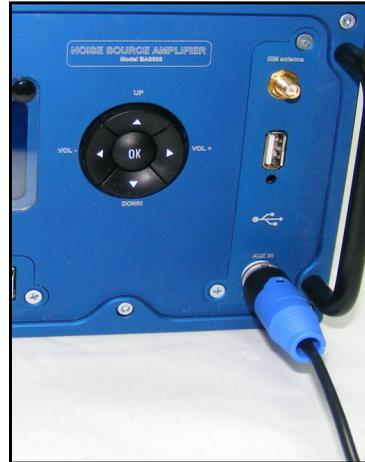
**FIGURE 3-6 CBL181 Connection to Power Amplifier**
