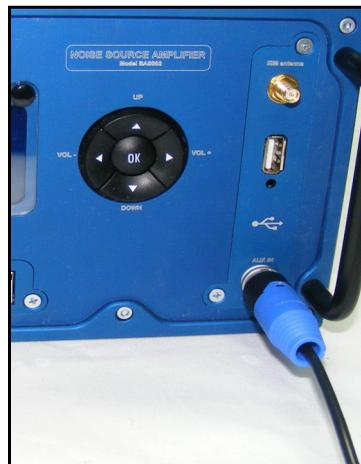
**FIGURE 7-9 CBL181 Connection to Power Amplifier**
