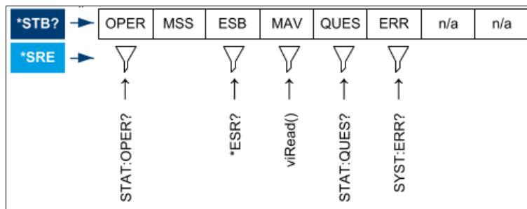
The STB corresponds to the EVENT part of a SCPI register, it indicates general instrument events. This register is cleared when it is read.
