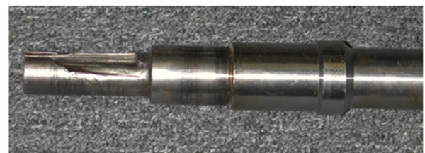
Figure 12: Picture of shaft from motor showing the shaft keyway wear.
