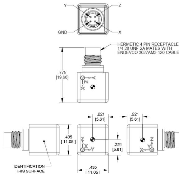
⊕ INDICATES LOCATIONS OF SEISMIC MASS
