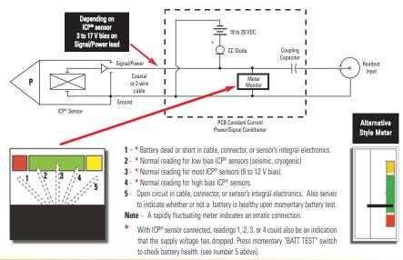
**GREEN** indicates normal operation. The cable and connections all have continuity and the sensor's integral electronics are turned on. The meter, which indicates sensor bias voltage, normally reads in the mid-range (9 to 12 V) for most ICP<sup>®</sup> sensors. A meter indication in the lower green is normal for low-bias sensors (3 to 6 V), such as seismic accelerometers and cryogenic pressure sensors. The meter registers in the upper green region for certain high-bias (15 to 17 V) sensors.
