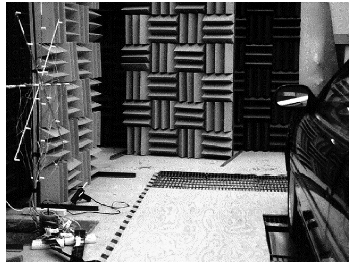
Figure 6: Photograph of the experimental setup used in the frequency domain temporal array method.
