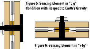
Condition with Respect to Earth's Gravity
