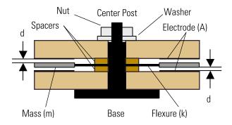
Figure 1: Sensing Element in "0 g" Condition
