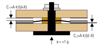
Figure 2: Sensing Element in "+1g" Condition
