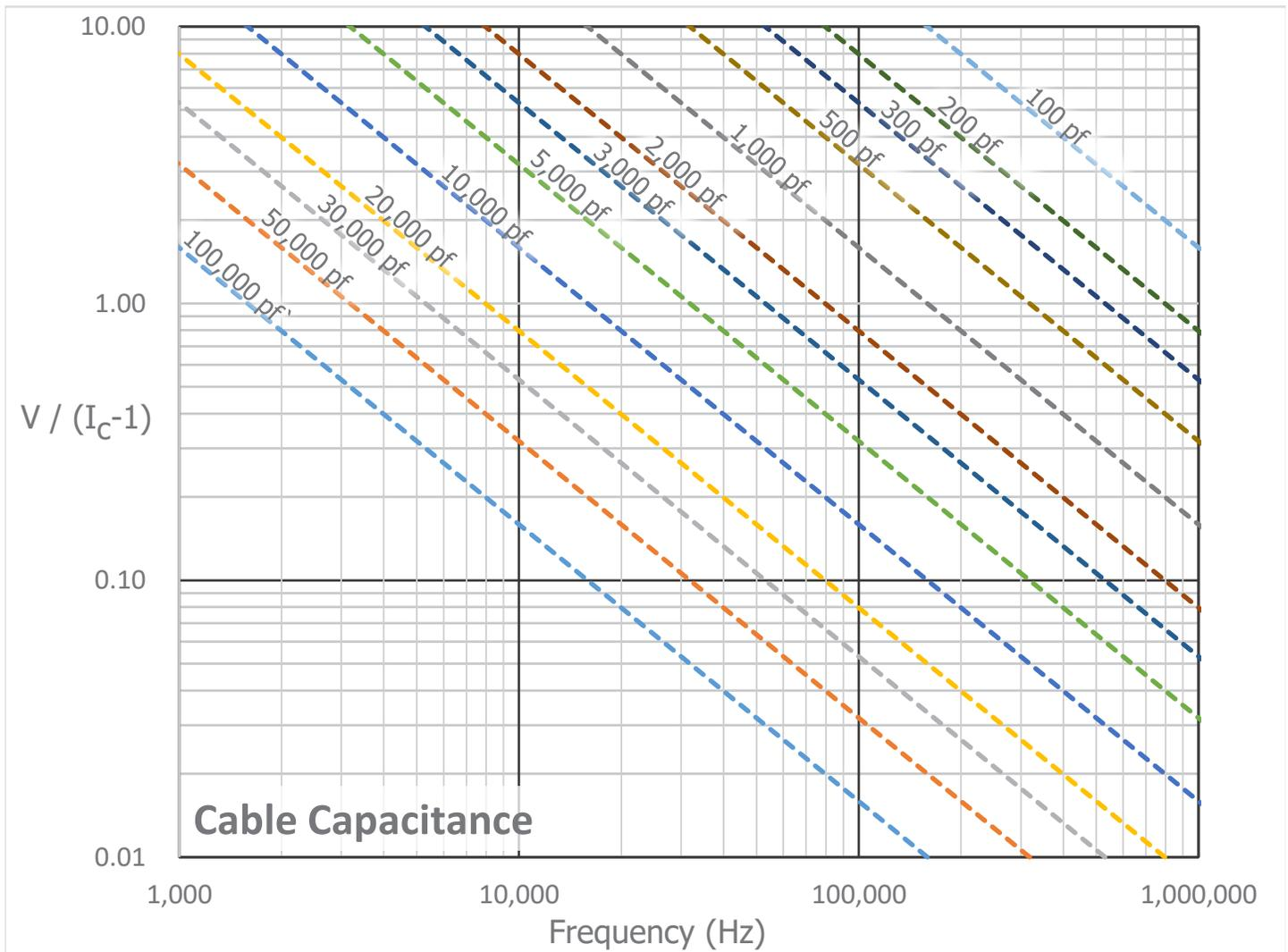
*Figure 4: Cable Driving Nomograph*
