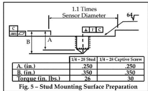
One last point worth noting regarding mounting involves surface preparation. In addition to surfaces being as flat as possible, clean and free of debris, and the mounting holes to be perpendicular, the mounting surfaces should be lightly coated with a lubricant. This coating aids in the transmissibility of the higher frequency vibrations and improves high frequency response of sensors. Silicone vacuum grease, heavy machine oil, or bees wax are commonly used.
