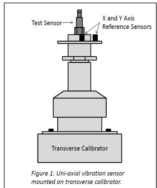
Figure 1: Uni-axial vibration sensor mounted on transverse calibrator.
