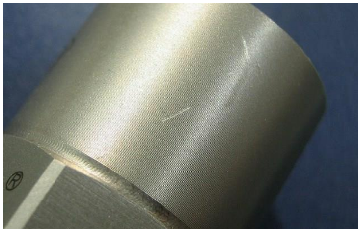
Figure 12 Unacceptable Scratches on Part Example
