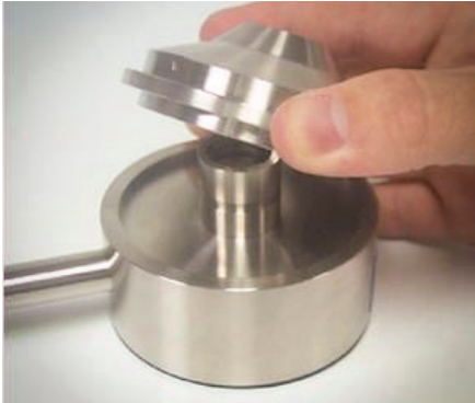
377A15 embedded in acoustic coupler for audiometry.
