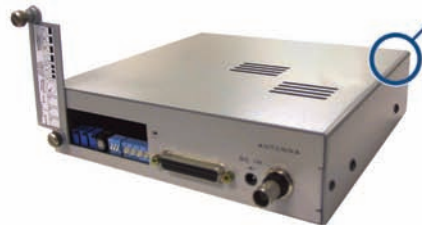
AT-4400 Receiver showing gain, offset, symmetry, gain, range, zero/added offset and output filtering options
