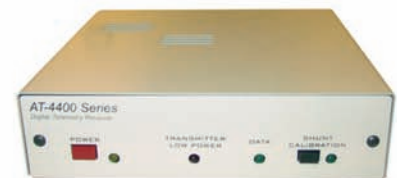
AT-4400 Receiver showing gain, offset, symmetry, gain, range, zero/added offset and output filtering options
