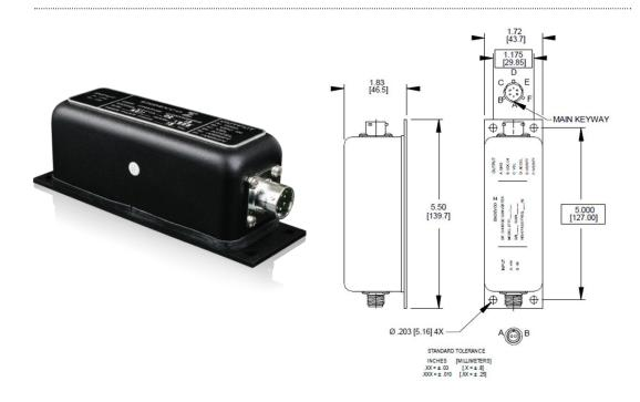
Model 2777A-XX-YY Differential Remote Charge Convertor (DRCC) is a low noise ruggedized device designed for use with differential piezoelectric transducers. This device converts the transducer's high impedance charge input to a low impedance voltage output. The acceleration output is also integrated to produce an AC voltage proportional to velocity output.
