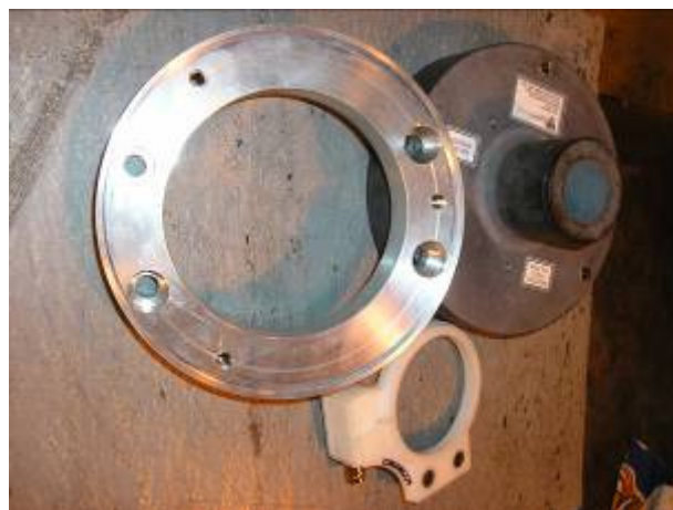
Figure 4 Adapter Plate, EFREM Transmitter “Top Hat” & Stationary Pickup Antenna
