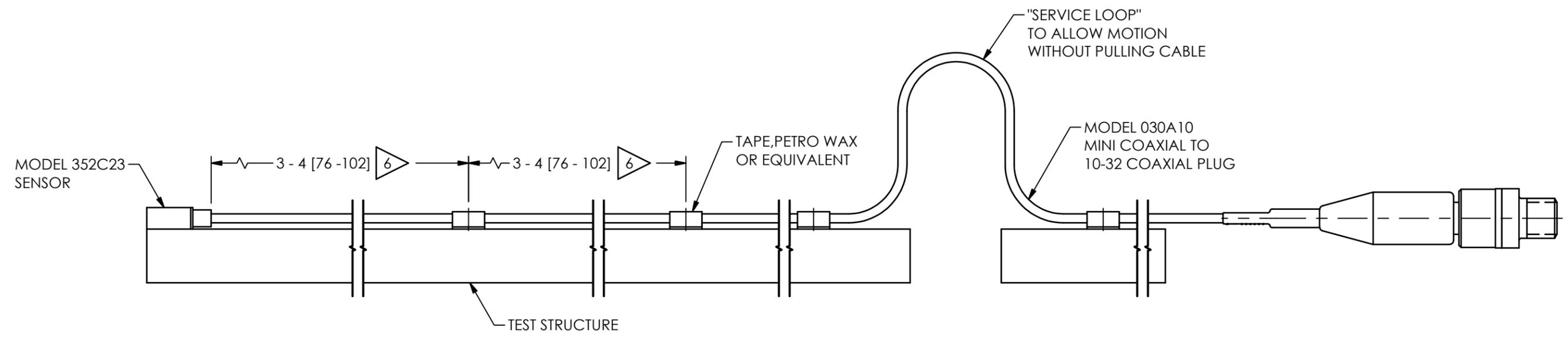
7.) TO AVOID UNNECESSARY DAMAGE TO THE SENSOR AND/OR CABLE, USE THE SUPPLIED REMOVAL TOOL (MODEL 039A37), A QUICK TWISTING MOTION WILL FREE THE SENSOR FROM THE TEST STRUCTURE
