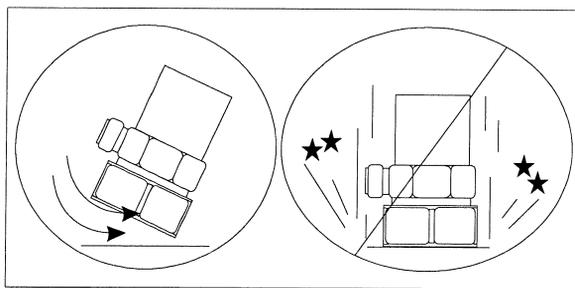
**Figure 7.** Magnet Mounting
