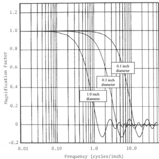
Figure 7: Frequency Response of Spatial Averaging Pressure Transducers
