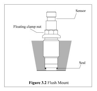
If thermal transients or diaphragm impingement are concerns, use the flush mount technique only when space or frequency response considerations preclude the use of the recess mount installation.
