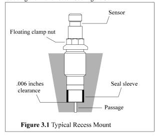
When using a recess mount, note that the length of the passage may limit the frequency range of the measurement. The effect the passage has is similar to that of an under-damped second order system, with the resonant frequency determined by passage length. The passage length thus limits pressure pulse rise time and may also cause passage ringing.
