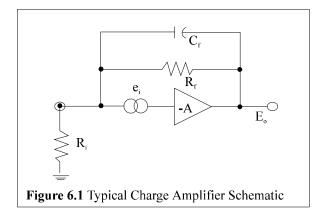
The feedback capacitor  $C_f$  comes into play only in the dynamic situation and its influence does not affect the steady-state situation. The voltage  $e_i$  is a DC offset voltage, usually very tiny (microvolts), that exists at the input gate of the MOSFET circuit. This minute leakage current exists in all real devices. As demonstrated in Equation 1, the steady-state (DC) output voltage  $E_o$  is:
