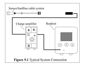
Before connecting the low-noise cable from the pressure sensor to the charge amplifier, be certain to ground the charge amplifier. This ensures that any excessive accumulated static charges across the sensor/cable combination are harmlessly discharged. If this precaution is not observed, the input FET of certain amplifiers may be destroyed. Press the ground button of the charge amplifier and adjust electrical zero if necessary.
