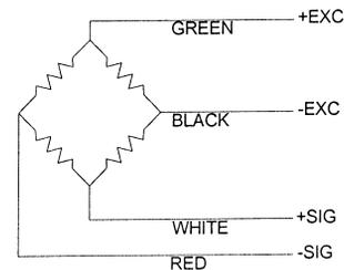
Figure 5 - S-Beam Load Cell Wiring Diagram
