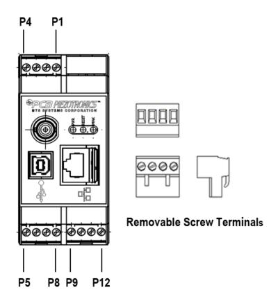
AC and DC input signals and power supply voltages could be hazardous. DO NOT connect live wires to screw terminal plugs, and DO NOT insert, remove, or handle screw terminal plugs with live wires connected.
