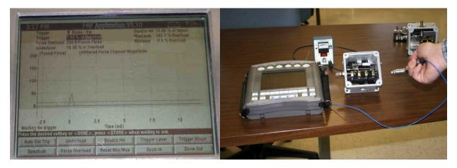
Figure 8: Impact test for mechanical vibration switches
