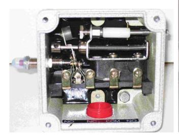
Figure 2: Traditional IMI Mechanical Vibration Switch
