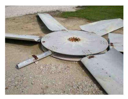
Figure 1: Catastrophic failure of a large fan due to high vibration
