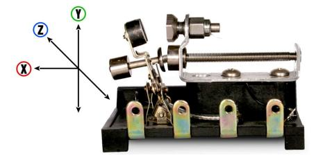
Figure 7: The sprung mass is sensitive to motion in three axes.
