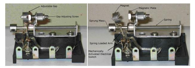
Figure 5: Armed mechanical switch mechanism with labeled parts
