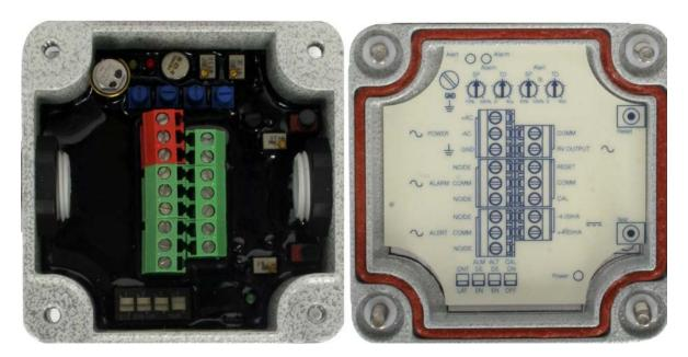
Figure 9: Traditional electronic vibration switch with potentiometer and DIP switch adjustments
